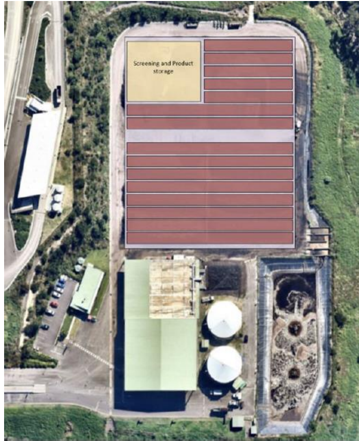
Figure 5: Proposed site plan detailing windrow layout similar to the original consent
