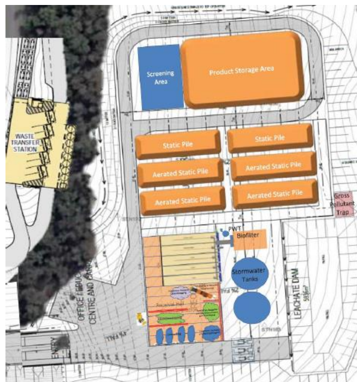
Figure 4: Approved modified site plan from DA/1940/2013/A
